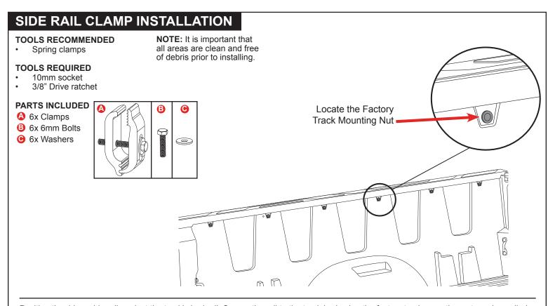
Position the driver side rail against the truck's bed rail. Secure the rail to the truck bed using the factory track mounting nuts and supplied 6mm bolts (B) and washers (C). Install 3 clamps (A) closest to the tailgate, closest to the cab, and middle hole, as shown below. Finger tighten the clamps, making sure the teeth properly engage with the grooves of the side rail. Repeat on the passenger side rail.
